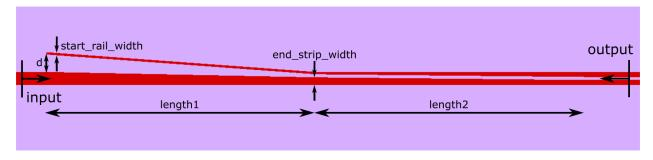
class picwriter.components.StripSlotMMIConverter( $wgt\_input$ ,  $wgt\_output$ ,  $w\_mmi$ ,  $l\_mmi$ , length,  $input\_strip=None$ , port=(0,0), direction=u'EAST')
