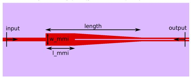
class picwriter.components.StripSlotYConverter( $wgt\_input$ ,  $wgt\_output$ , length, d,  $end\_strip\_width=0$ ,  $end\_strip\_width=0$ ,  $end\_strip\_None$ , port=(0, 0), direction=u'EAST')
